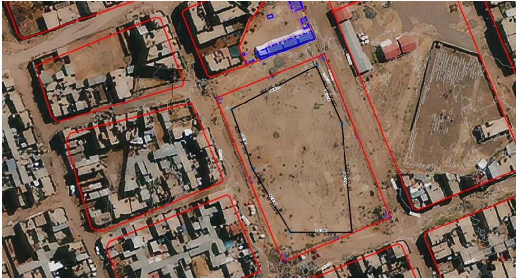
Figura 16.-Poligonal de control horizontal
