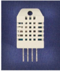
Capacitive-type humidity and temperature module/sensor
